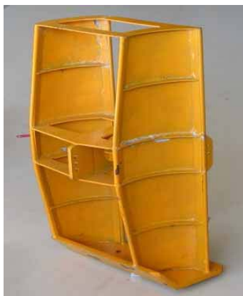
Figure 10 Bi-plane otter board construction and design for vessel 1000PS engine
